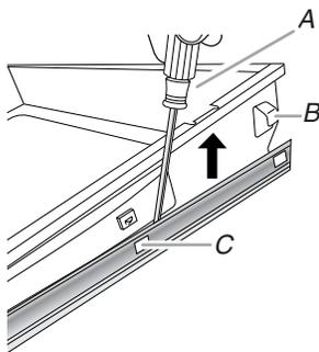
3. Repeat Step 2 on the other side. The warming drawer or premium storage drawer is no longer attached to the drawer glides. Using both hands, pick up the warming drawer or premium storage drawer to complete the removal.
