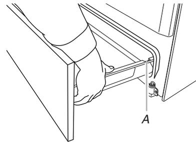
2. Lift up the front of the drawer and pull the drawer out.
