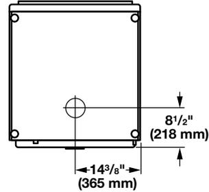
**NOTE:** Most installations require a minimum of 6" (152 mm) clearance behind dryer for exhaust vent with elbow. See "Venting Requirements."
