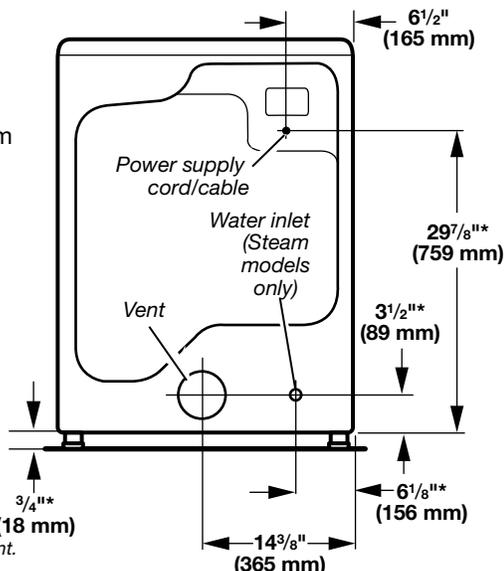
**NOTE:** Most installations require a minimum of 5" (127 mm) clearance behind dryer for exhaust vent with elbow. See "Venting Requirements."
