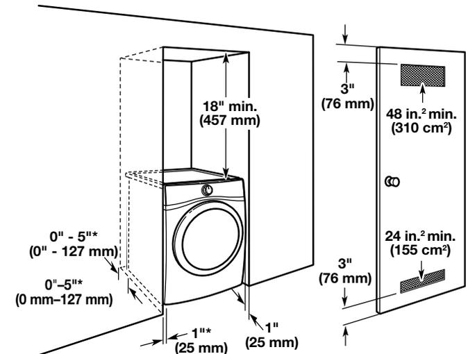
\*0" (0 mm) spacing is allowed for straight-back venting only. For steam models only, inlet hose must not be kinked.
