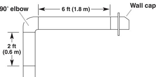
The following example falls within the maximum recommended vent length of 35 ft (10.7 m).
