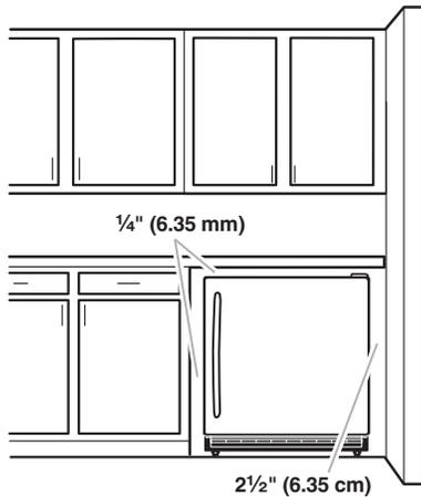
To ensure proper ventilation for your refrigerator, allow for a 1/4" (6.35 mm) space on each side and at the top. When installing your refrigerator next to a fixed wall, leave 2 1/2" (6.35 cm) minimum clearance on the hinge side to allow for the door to swing open.
