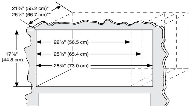
\*With flush receptacle, or with non-flush receptacle located in upper right or upper left corner of cutout.
