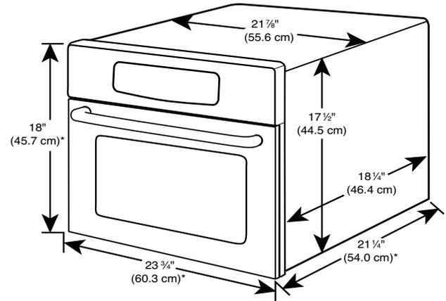
\*Measurements include front facing of microwave oven. Depth measurement also includes door handle.
